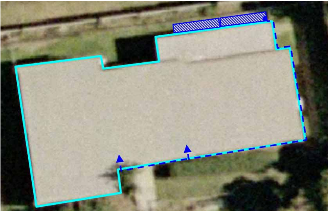
Roof catchment 2 x 5kL Rainwater tank footprint Rainwater reuse pipeline
