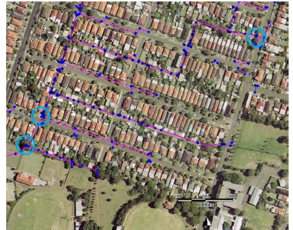
Stormwater infrastructure and location of observed base flows in Ashbury (circled in blue). Blick and Campbell ovals can be seen at the bottom of the photo
