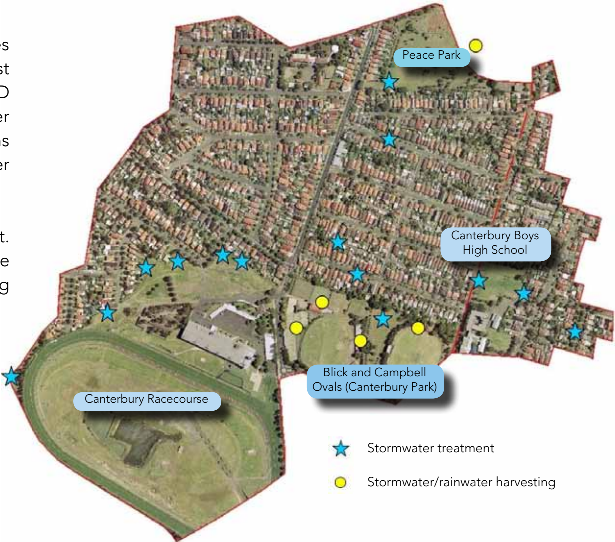
Ashbury Subcatchment showing the location of sites that are potentially feasible for WSUD features; these have been identified through the OurRiver project.
